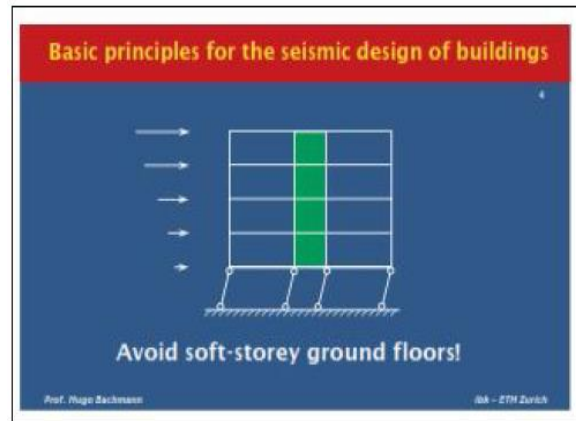
Figure. 2 Seismic Conceptual Design and Capacity Design
