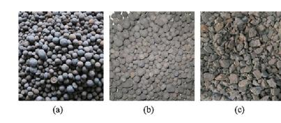
Numbers with a thin border: Figure 1. partly round shale ceramist S1 (a), squished shale ceramist S1 (b), squashed shale ceramist S1. Compressive strength as a function of wall thickness
