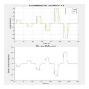
The adaptive gains also stay constant as a result of the perfect modelling of the ideal system. Additionally, the system is able to account for the presence of a fault. If the elevator efficiency is set to 0.7, the aircraft responds in the following manner.
