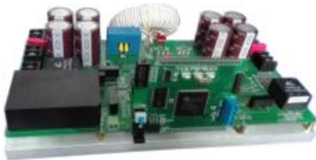
Fig. 9 The experimental prototype of the proposed switched-capacitor bidirectional DC-DC converter.
