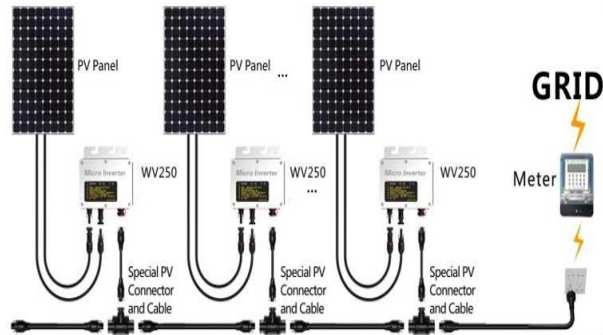
Fig.3.1: Pv panel fed micro-inverter
